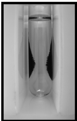
Fig. 7. Induced MAG-PANI separation from the reaction medium by the application of a magnetic field. MAG-PANI support is displaced towards the tube walls.
